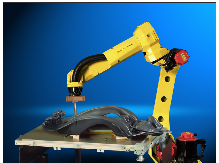
Plastic part material removal
